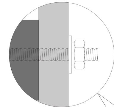
If the backing wall is thin and construction can be performed on the another side of the back wall, please use nuts and washers to fix the stud bolts on the back wall, so that the signage can fix on the backing wall more secure.
